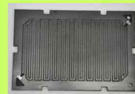
100 cm 2 multi-channel serpentine flow field plate
