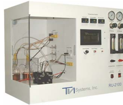
TVN Systems' PEMFC Test-Stand
